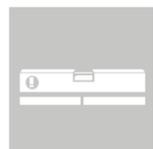
The bearing surface for the tile should be perfectly plane – without cracks, impurity, cavity pockets, void pockets. Installation surface should be dry, hard (durable), free from impurity.
